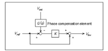
Fig. 4 Block diagram of inverter control
