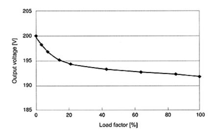
Fig. 8 Output voltage with regard to load factor
