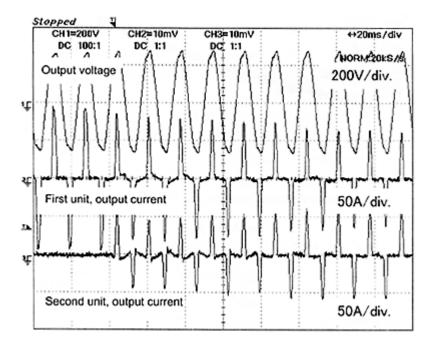
Fig. 15 Experimental results (when the rectifier is loaded, with a second unit introduced)
