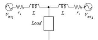
Fig. 1 Parallel connected model of UPS
