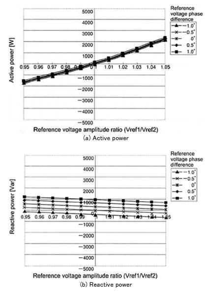
Fig. 13 Active and reactive powers of the cross current (  $r_{_S}$  = 0,  ${\cal K}_{_L}$  = 2.5)
