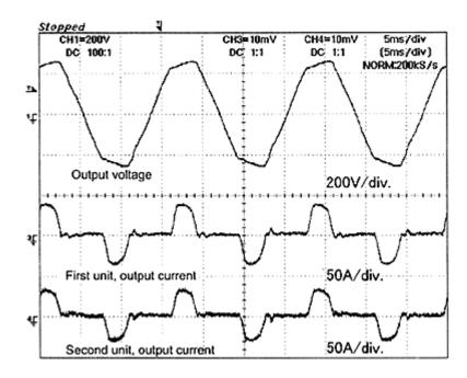
Fig. 14 Experimental results (when the rectifier is loaded)
