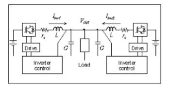
Fig. 3 Parallel connected model of UPS used in the simulation
