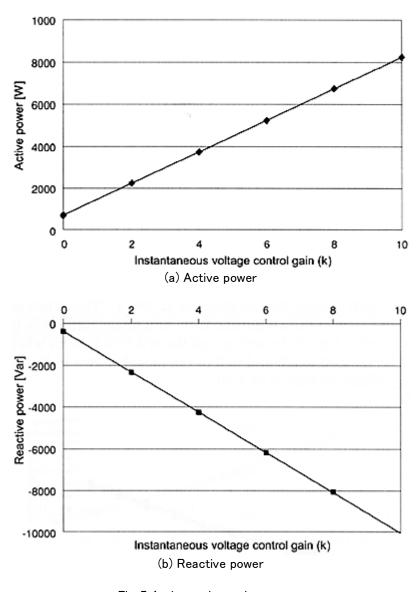
Fig. 7 Active and reactive powers of the cross current with regard to the gain  $% \left( {{{\mathbf{F}}_{i}}^{T}} \right)$
