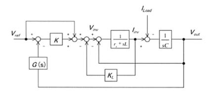
Fig. 12 Block diagram of parallel run control of UPS
