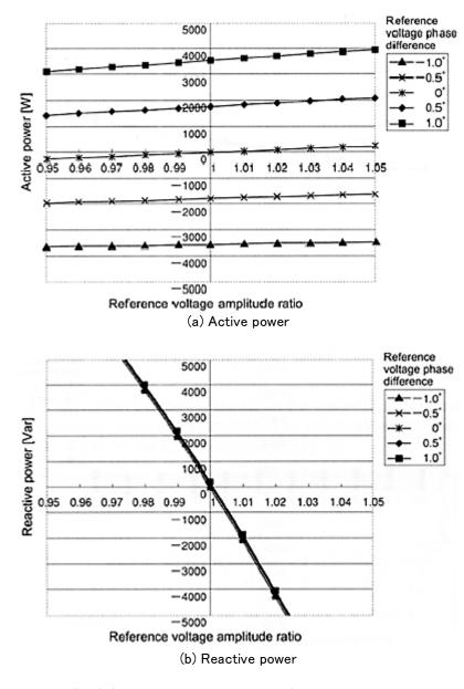
Fig. 6 Active and reactive powers of the cross current with regard to voltage ratio and amplitude difference
